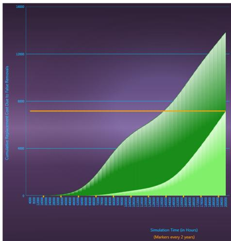
Fig. 13. Extra cost due false removals over time for the Alternative Design 2 model.
