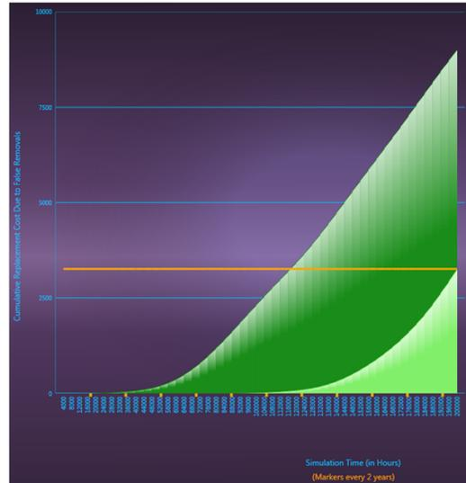
Fig. 17. Extra cost due false removals over time for the Alternative Design 3 model.
