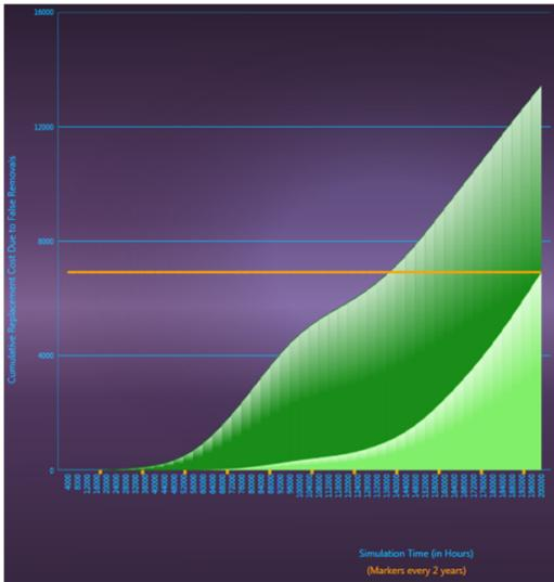
Fig. 7. Extra costs due false removals over time for the “reference” model.
