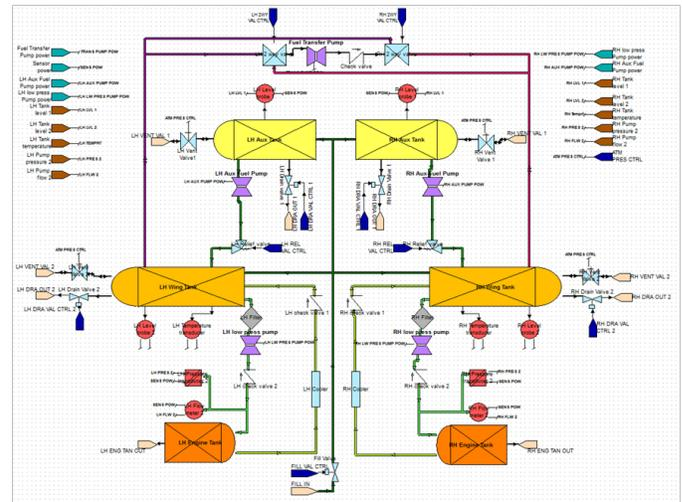
Fig. 2. Design of the fuel system model in eXpress<sup>TM</sup>.
