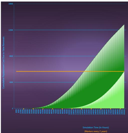
Fig. 8. Extra costs due false removals over time for the Alternative Design 1 model.
