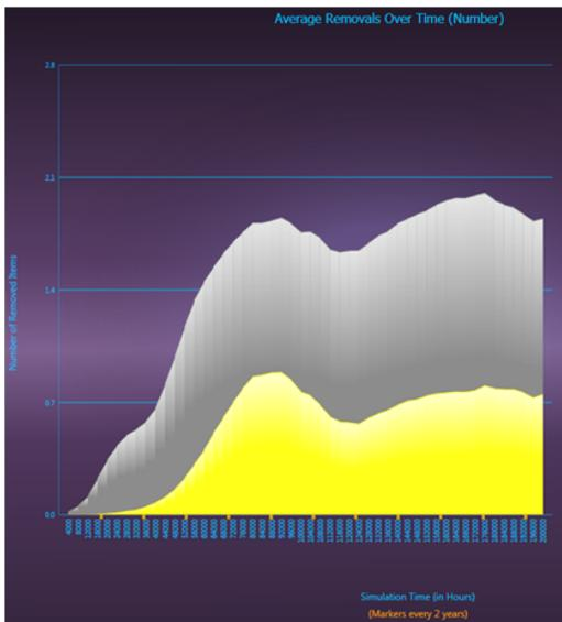
Fig. 16. Average removals over time for the Alternative Design 3 model.
