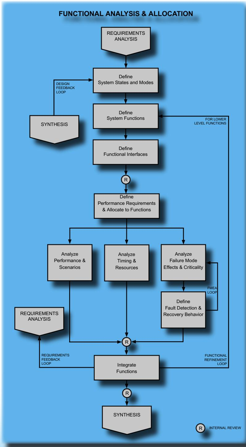
As the Functional Analysis begins, the analyst must define various attributes of the system such as System States and Modes, System Functions, and Functional Interfaces. The activity may periodically be influenced by design feedback and functional refinement feedback. These feedback inputs shouldn't perturb the process but rather enhance the synergy necessary to flush-out important system engineering / diagnostic issues.
