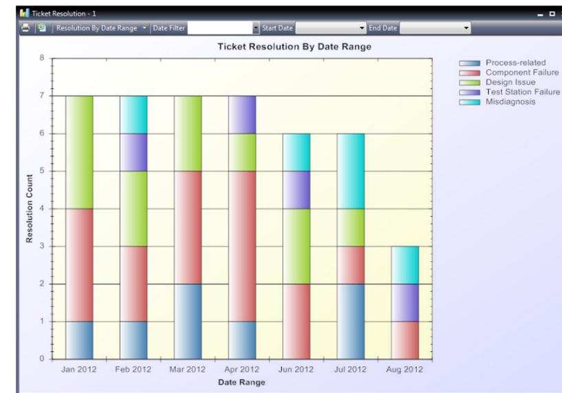
This sample report shows ticket resolution by month, with the number of resolved tickets categorized by user-specified resolution categories (in this example, the categories are: Process-related, Component Failure, Design Issue, Test Station Failure & Misdiagnosis).
