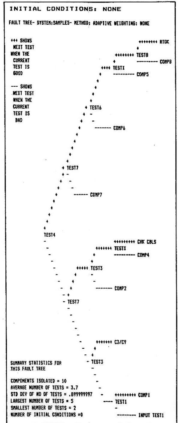
Figure 3. Sample Fault Tree
