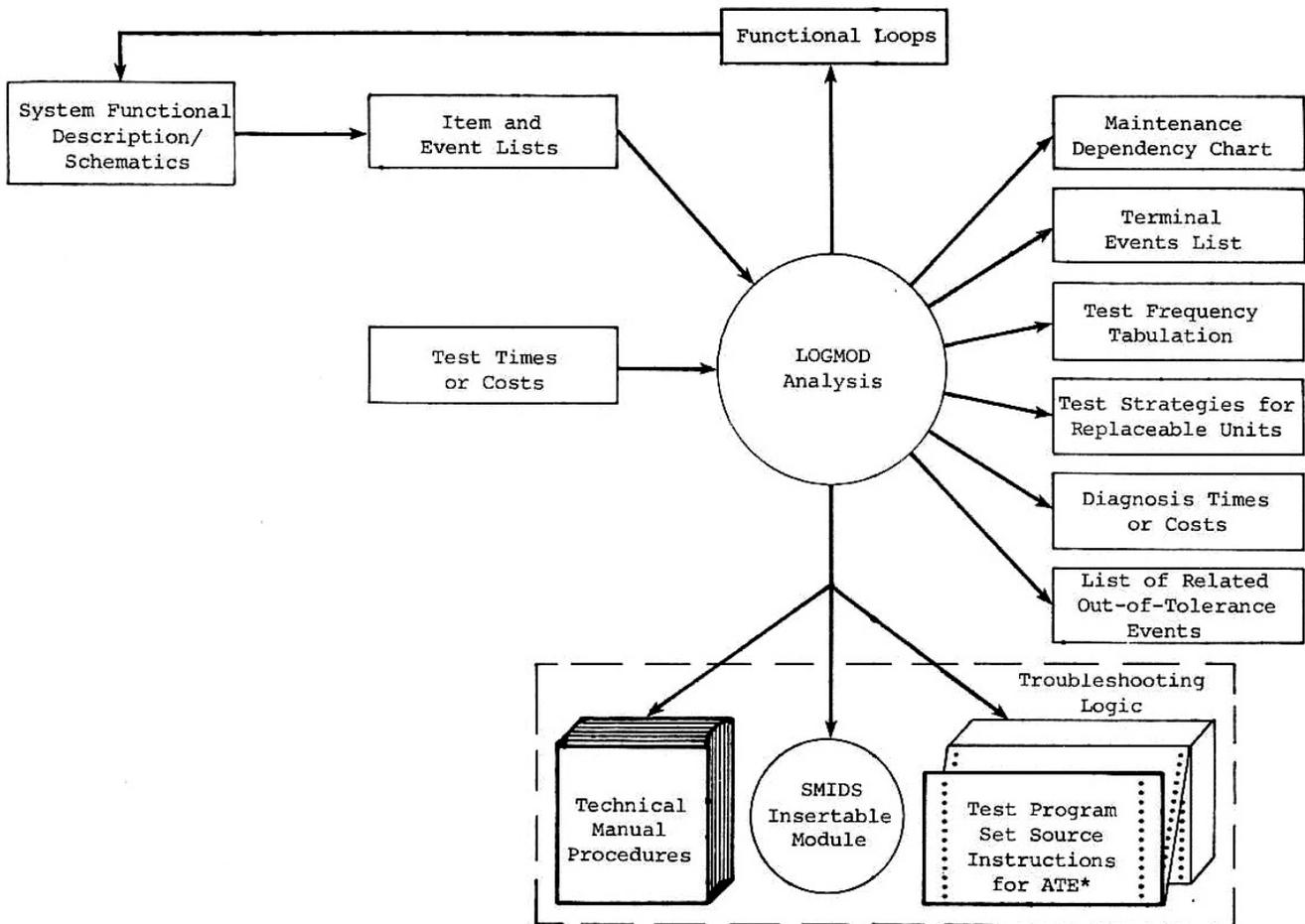
Figure 10. LOGMOD INPUTS AND PRODUCTS
