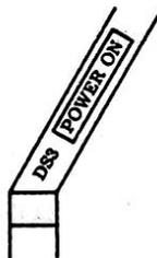
When the indication is observable from outside of the equipment, the panel nomenclature (if any) for the indicator shall be illustrated by a black-line box around the panel nomenclature.
