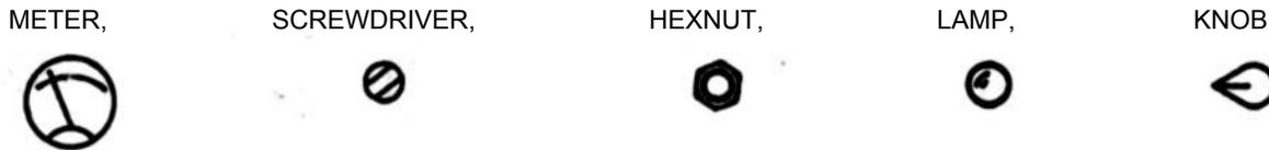
The adjustment or control marked nomenclature and its appropriate symbol shall appear in the hardware area representative of the hardware upon which it is located. The relationship of an adjustment or control to the proper part shall be illustrated by means of a dashed-line connection.
