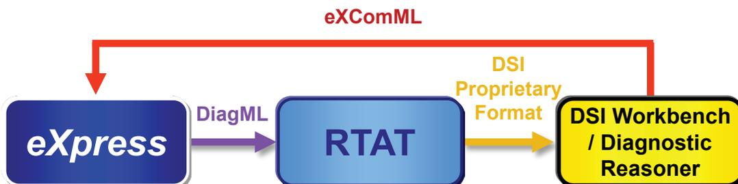
**Turn-key Diagnostics** – Deploy static or dynamic diagnostic procedures from *eXpress* in DSI Workbench or one of DSI's other diagnostic reasoners.
