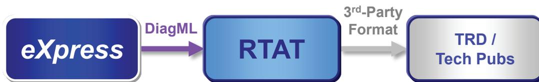
**Test/Diagnostic Documentation** – Use test definitions and diagnostic sequences generated in *eXpress* to develop TRDs (Test Requirements Documents) and written test procedures.
