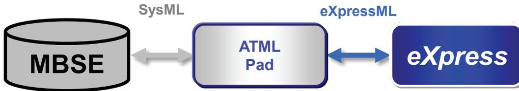
**Model-Based Diagnostic Engineering** – Jump-start **eXpress** modeling using design data from MBSE databases (such as MagicDraw or Capella); then record details of the diagnostic design back into SysML models.
